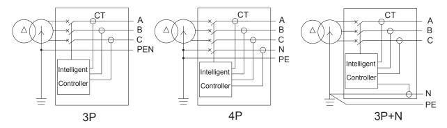
Grounding current: Measure current between phase line and neutral in a TN-S system, measure in the Neutral - earth link of the LV transformer (shown below), when there is a grounding fault, PE line will generate current, causing fault determined.
