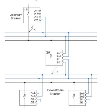
Zone-selective interlocking (ZSI) has multiple classified protection system which is designed to minimize the faulty impact on whole electrical distribution system by reducing the time it takes to clear the fault and maintaining system coordination. This function is suit with short circuit and ground fault protection (I<sup>2</sup>t is set to off)
