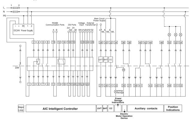
Note: (1) If CC, SHT and M are using different control voltage, they should connect to different power source.
