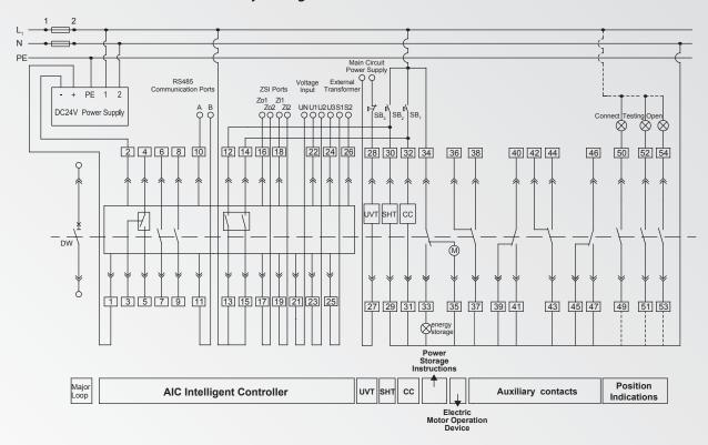
Note: Set the first set of programmable contact (12 # , 13 # )"remote open" and pair with a SHT; set the second programmable contact (14 # , 15 # ) to "remote close" and pair with a CC; then use the controller to send out signal for remote control.
