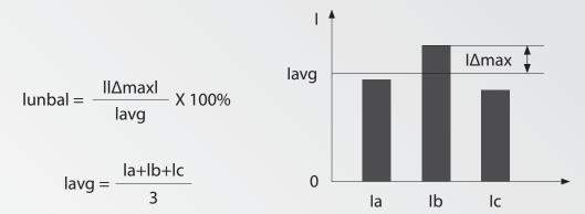
In the equation, lavg: la,lb,lc 3 phase average current (RMS).  $I\Delta max$ : maximum difference of each phase and lavg.
